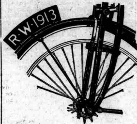
The Rudge-Whitworth Motor-Cycle Fork. geared machine, the Tourist Trophy type, the "free-engine" model, and the "Rudge-Multi."
